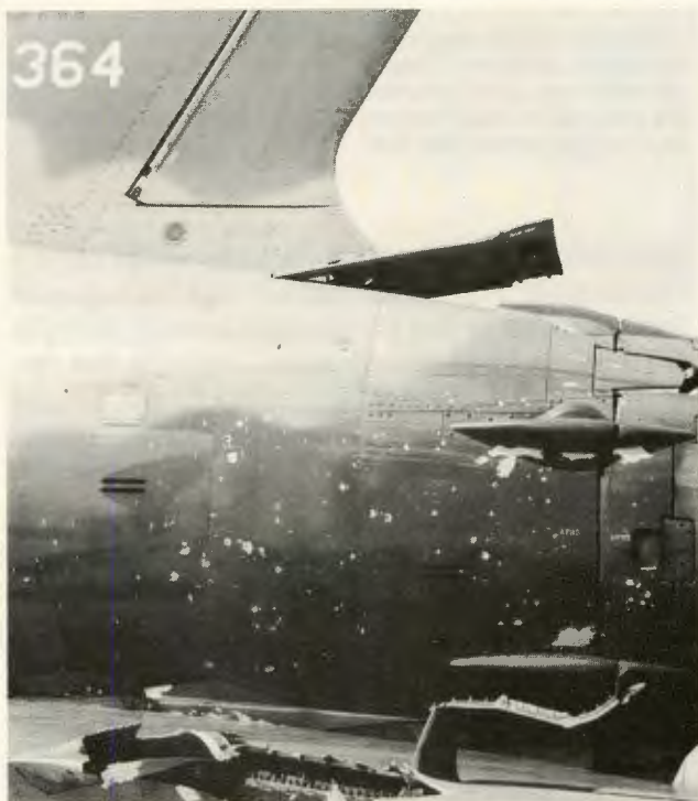
Battle damage? Not really. This aircraft flew through the CBU pattern of the flak suppression flight. The strike flight briefed to release at 5,000 feet and stay close to the flak suppression flight. The flak suppression flight briefed CBU opening at 10,000 feet. Neither flight knew of the other flight's plans.
