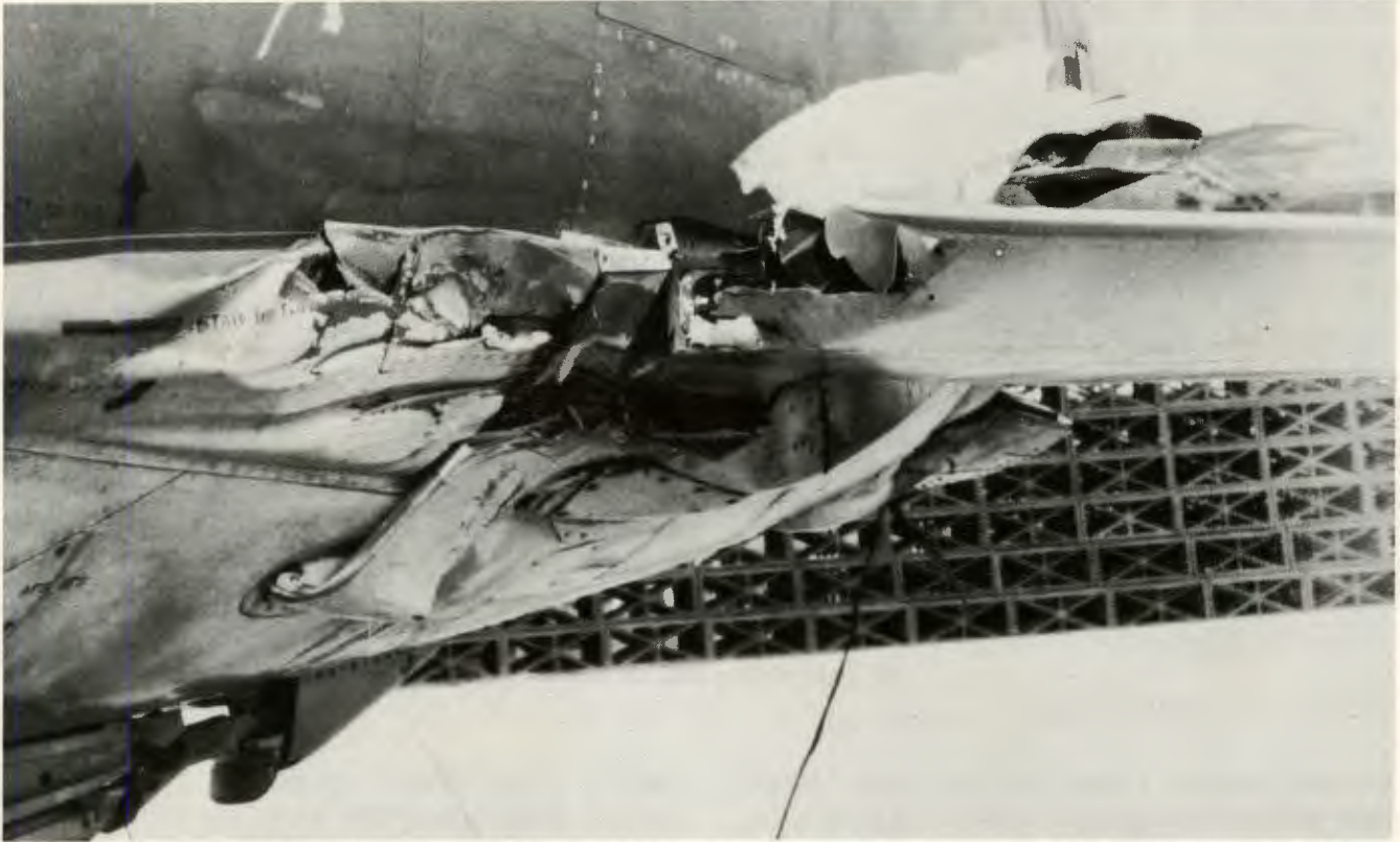
Route Pack VI strike. This was a normal release with good parameters, but one bomb had no fins. The wingman saw the fins come off on the way inbound; however, no one in the flight recognized the potential problem. When released, a bomb without fins tumbles end-over-end. Even low-speed jettison should include the rack when possible.
