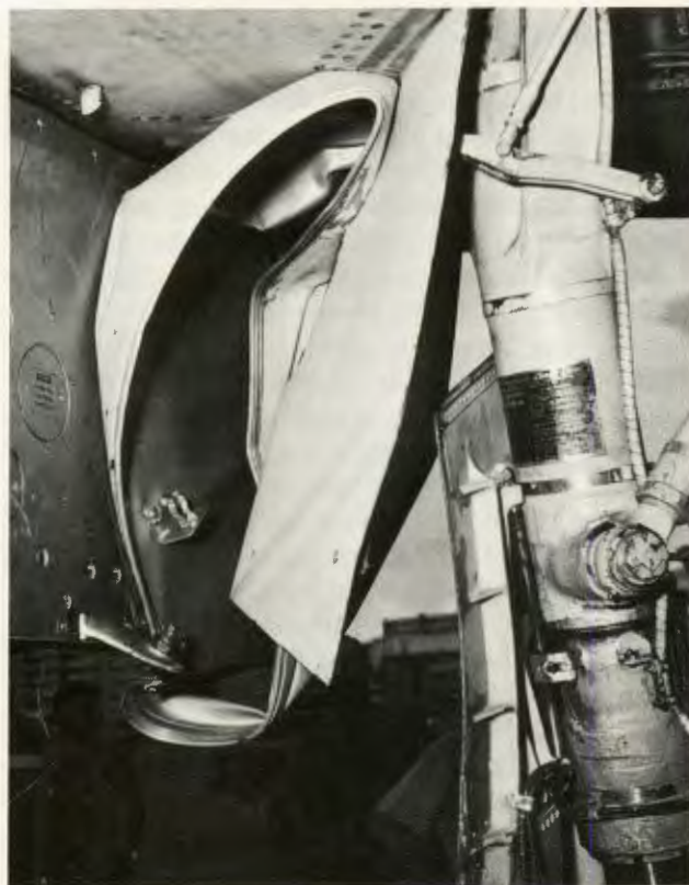
Over-G: Partially filled fuel tanks can fail in many ways when exposed to excessive G-loading. This tank rolled up to the inside of the main wing pylon. Afterwards, during landing gear extension, the pilot had to apply increased G's so the gear would crush the tank and fully extend and lock.
